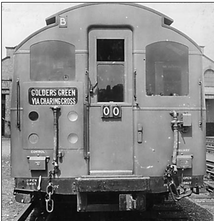
Figure 8 (left): The 1926 front end was also altered so that the marker lights and tail light were grouped into a box on the offside of the cab and the destination signs were moved from the original position over the end door to the offside box. The train set number was now positioned on the front door just under the window, instead of being higher up. The emergency lighting jumper is now low down, with the socket under the marker light box. Photo: LT Museum.
