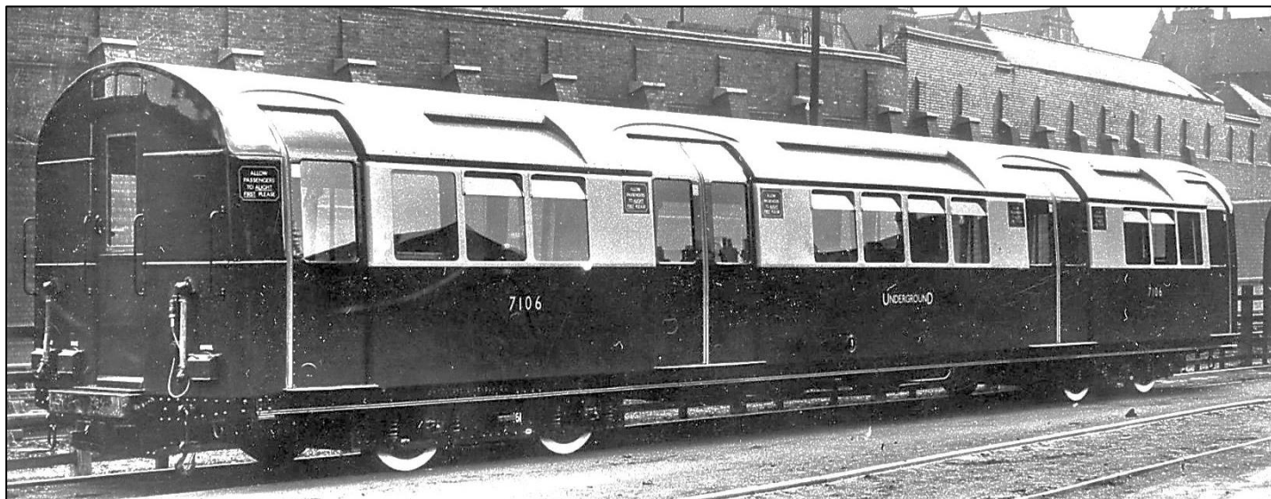
Figure 14 (below): A 1934 Met. Cammell motor car at Cockfosters depot. This was the final design of the LER's Standard stock and was virtually identical to the 1931 design. The line name on the side of the car was a short-lived idea introduced shortly after London Transport was formed in 1933. Photo: LT Museum.
