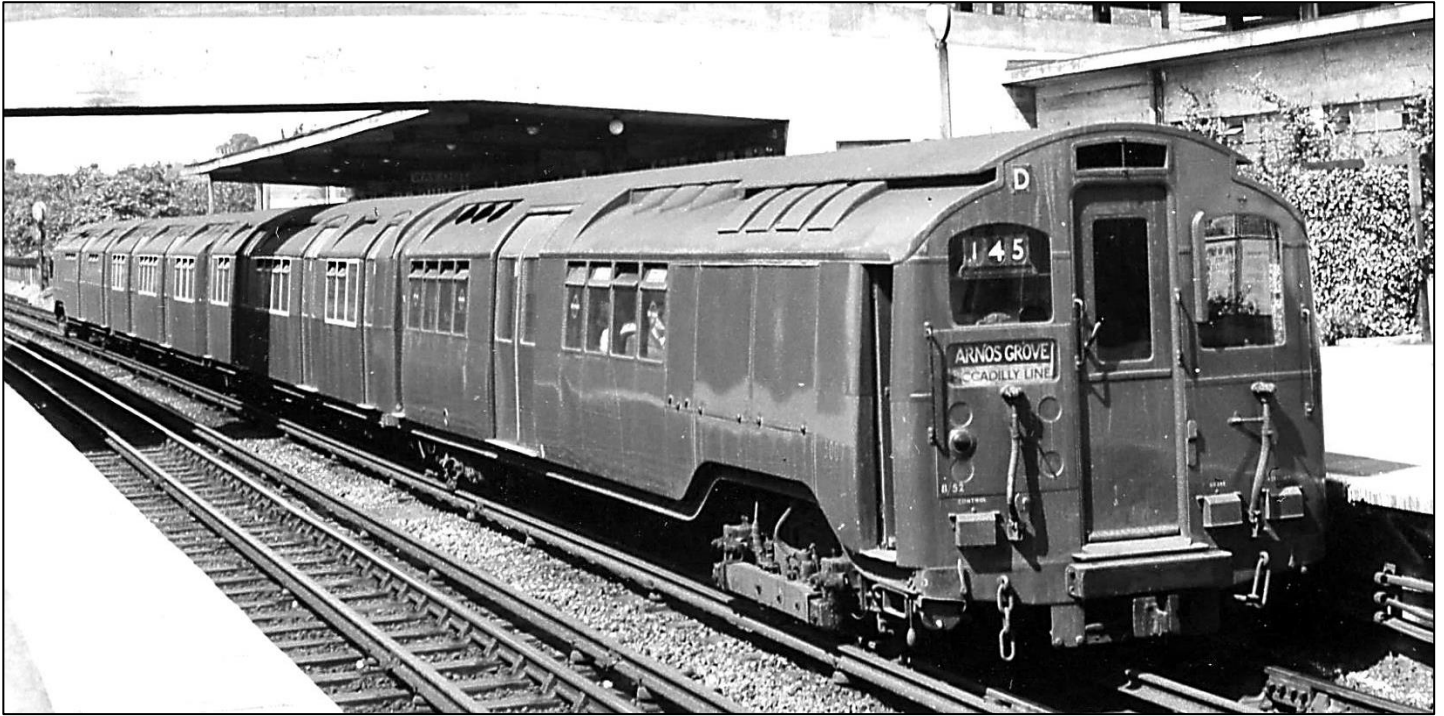
Figure 11 (above): A 4-car Piccadilly Line train at Sudbury Town about 1953. The leading car is a 1929 motor car by UCC and has the typical curved lower panels and straight gutters of this builder. Note that the roof ventilation louvres have been covered to reduce water ingress. Note also that the train line angle cock switch has disappeared, having been replaced by an internally mounted “pneumatic interlock” on EP brake equipped trains. From early 1952, cars coming out of Acton Works after overhaul lost all the cream paintwork and were perhaps poorer for it. A modification seen here is the provision of a window wiper for the driver. Drivers didn’t get window wipers until the introduction of the 1931 Stock. Photo: B.R. Hardy Collection.
